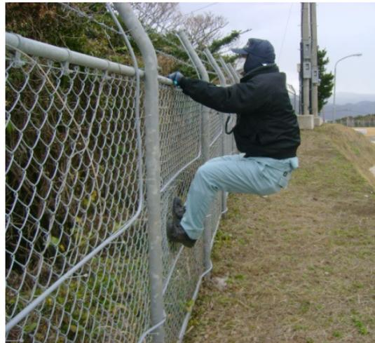
Initially we try a very simple algorithm that measures the change in light and, when the change gets too big, sounds an alarm. We test our system and find we have a 99.5% probability of detecting a person attempting to breach the perimeter. But when we test the NAR, by letting the system run continuously for several days, we find that our sensor generates about 10 nuisance alarms each day. This is a very high figure so we investigate and find the system alarming on all
