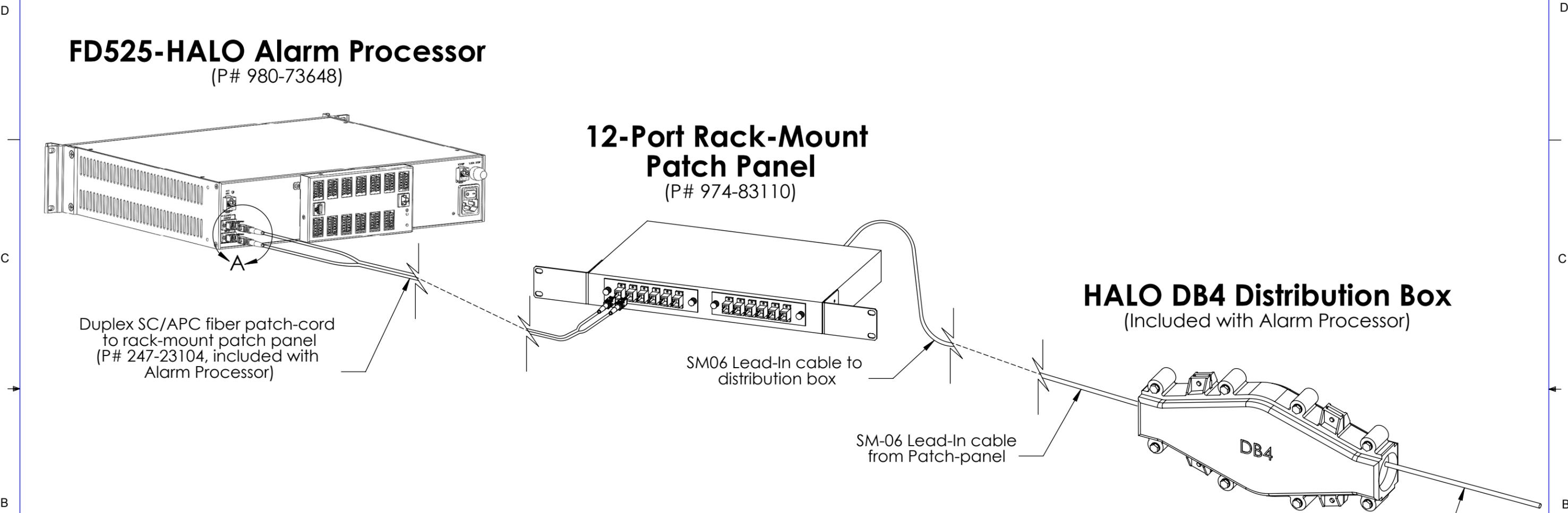
Duplex SC/APC fiber patch-cord to rack-mount patch panel (P# 247-23104, included with Alarm Processor)
