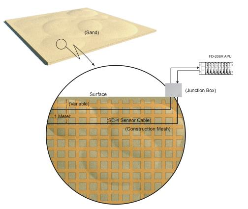
Figure 3 - Protecting against tunneling-type intrusions
