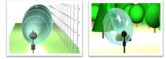
Figure 5: Avoid areas that will interfere with proper operation of Bi-static detection zones.
