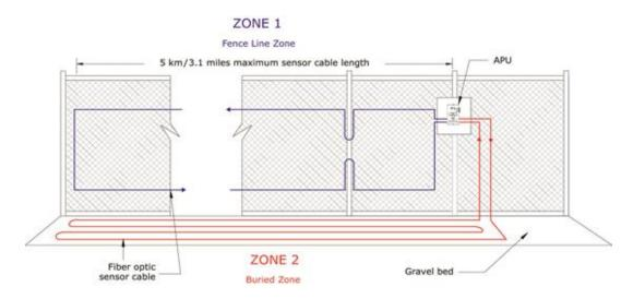
Figure 1: Field mounted APU head-end with dual -zone configuration, fence mounted sensor cable & buried zone.
