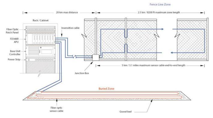
Figure 2: Rack-mounted APUs located in remote facility, with full capacity of up to 8 independent zones.
