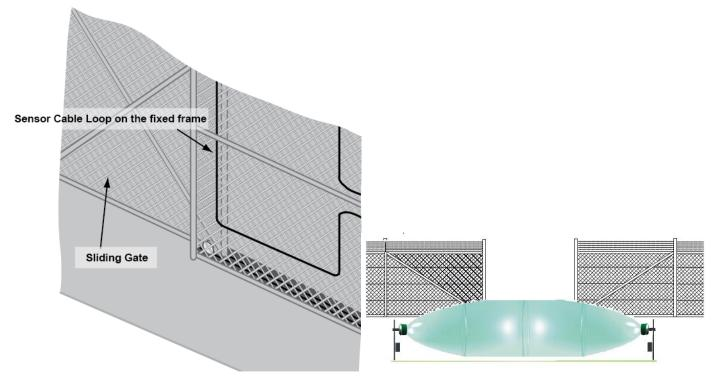
Figure 17: Sensor cable deployment on a sliding gate
