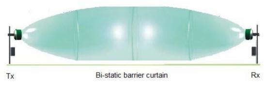
Figure 4: Volumetric microwave barrier curtain models range from 50 m to 500 meters.
