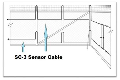
Figure 3: Double fiber cable installation, with dual-zone cross over in a high-security fence corner.
