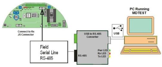
Figure 11: RS-485 to USB connections to PC
