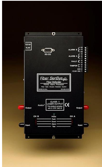
Connect one end of the cable being used to detect breaks to the output port on FD322; connect the other end to the input port (on the same side).
