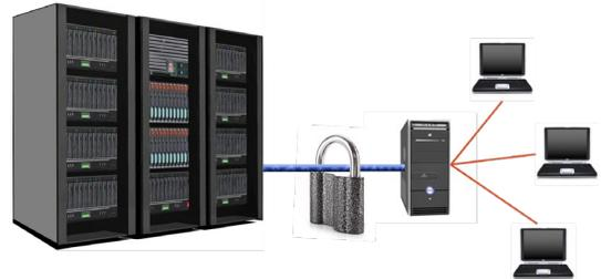
Data encryption is a standard way of protecting information but given enough time encryption can be defeated. Fiber SenSys, Inc., offers **SecurLAN**, an intrusion detection system designed to protect data networks at the **physical layer**. **SecurLAN** monitors the data cable for vibrations caused when an intruder tries to cut or tap into the network cables. Unlike encryption, **SecurLAN** cannot be “cracked.”
