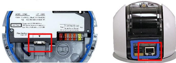
Figure 8: LD204S Main Ethernet port (L) and maintenance port (R) location
