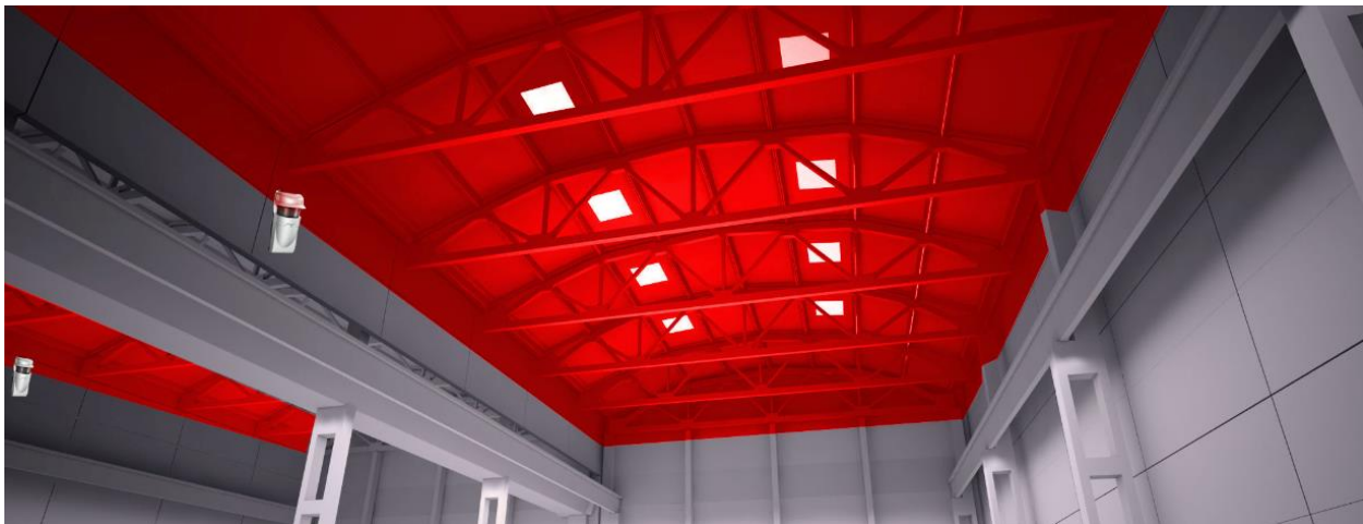
Figure 13: LD308SH in horizontal mode protecting skylights from intrusions using Indoor Ceiling/Wall protection mode
