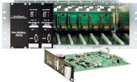
This rack-mounted APU is equipped with TCP/IP (via XML messaging) and supports sensing cable up to 5km; with insensitive lead-in cable up to 20km for remote APU deployment. The RK-348 rack housing holds up to eight FD348R APUs.
