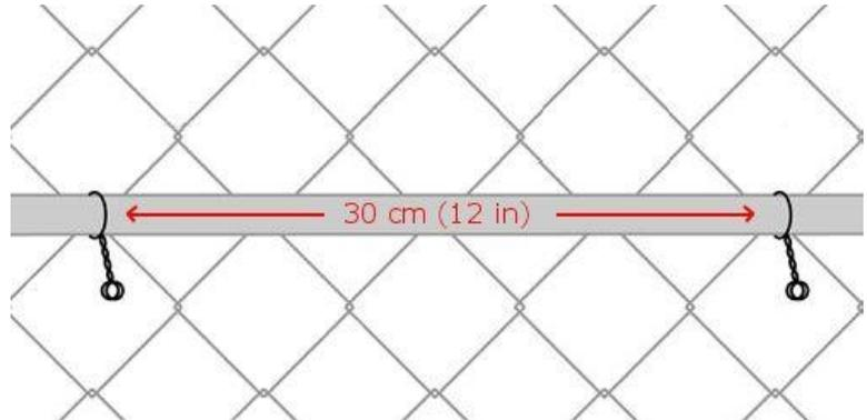
2. Use only stainless steel wire ties to attach conduit.
