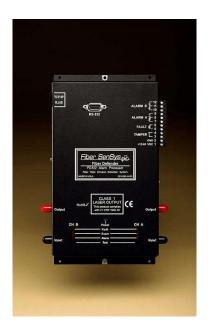
The fiber-optic sensor is especially applicable to areas frequented by severe thunderstorms and lightning because the optical fiber cable/conduit will not conduct electrical discharge back to the APU, and because the sensing fiber is unaffected by EMI resulting from lightning strikes.
