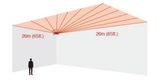
Powerful PC-based tuning software allows precise detection areas.
